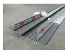
Remove the protective film tape of the required metal water stop for element wall's controlled crack joint flashing (however, do not remove protective film tape with FRANK logo as this tape reduces the bond between the concrete and the metal plate) and afterwards place metal water stop at empty end of the element wall already erected (clean off adherent grit or other contaminations from adhesive surface).
