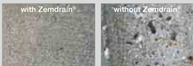
Picture 1: Visual difference between concrete walls produced with Zemdrain® and without Zemdrain® at the walls of the wastewater treatment plant Offenburg after 10 years of operation.
